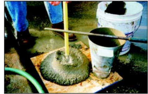
Typical Slump Test
